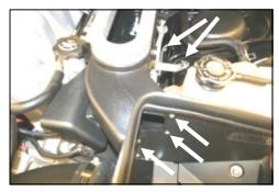
**12.** Install the hood scoop into the **CAD** using three 8-32 x 3/8" button head screws (#14), and three #8 flat washers (#15), leave loose. Install the L-bracket (#23) over the stud on the fender, and bolt it to the hood scoop using one 1/4-20 button head bolt (#12), and 1/4" flat washer (#13). Replace the factory nut on the stud, adjust for fit, and tighten all bolts, nuts, and
