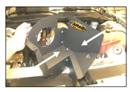
**7.** Assemble the two Cool Air Dam (CAD) panels (#2, #3) using five 6-32 x 5/16" screws (#16), #6 flat washers (#17), and 6-32 keps nuts (#18). Apply the Airaid Decal on the Panel as shown.
