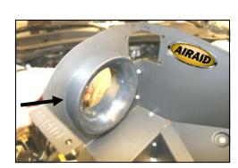
**8.** Next, install the filter adapter (#5) using three  $\frac{1}{4}$  - 20 x  $\frac{1}{2}$ " button head bolts (#13), and  $\frac{1}{4}$  flat washers (#14).
