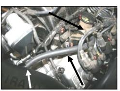
17. If you are working on a 6.1L, skip to step #18. If you are working on a 5.7L, install the Breather Hose, Barbed Fitting and Elbow from the valve cover to the Airaid Intake Tube as shown. ( See exploded view for detail ) Re-install the engine cover.
