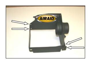
**5.** Assemble the Quick Fit Panels (#2, #3) using four 6-32 x 5/16" screws (#5), #6 flat washers (#6), and 6-32 keps nuts (#7). Apply the Airaid Foil Decal onto the Panel as shown.
