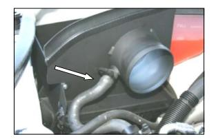
7. Re-install the breather hose and speed clamp (#8) onto the nipple on the Quick Fit Panel. If you are working on a 6.1L, install the 1/2"x 90° elbow (#9) from the breather hose to the nipple on the Quick Fit Panel.
