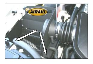
**6.** Install the Quick Fit Panels by sliding the four tabs on the back of the panels into the factory airbox base, and then into the factory intake tube. Relatch the two factory clips into the slots on the front of the Quick Fit Panels. Tighten the hose clamp on the factory intake tube.
