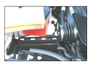
**4.** Remove the factory air filter from the airbox base.
