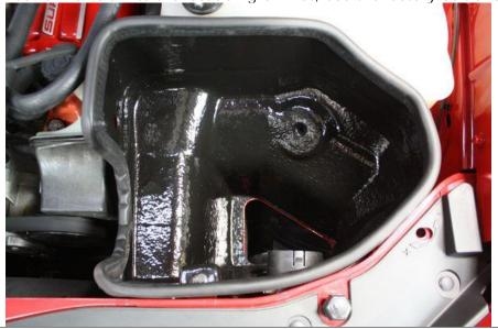
CHALLENGER: route the factory inlet tube through the heat shield, onto the headlight. Use the supplied FOAM GASKET to seal the Fresh Air Inlet tube to the heat shield.
