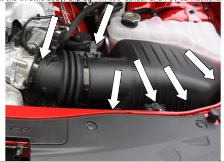
4 CHARGER: Unclip(squeeze) the 4 retaining clips in the air box holding the Fresh Air inlet to the box and remove the lower air box.
