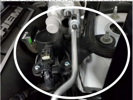
**TIP**: The PCV line twists at both ends. Twist and connect to the PCV connection on the solenoid from the valve cover
