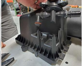
**6** Use the supplied hardware and bracket to mount the solenoid to the bracket as shown.
