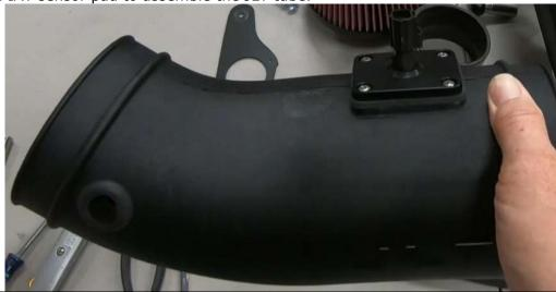
**5** Using a utility knife, remove the 3 tips of the plastic welded rivets and remove the PCV solenoid.
