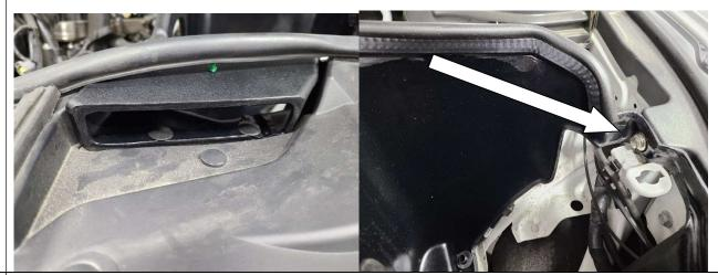
Lower air filter down into the airbox first, then with the silicone reducer on the tube with clamps loose, connect the tube and air filter then slide onto throttle body.
