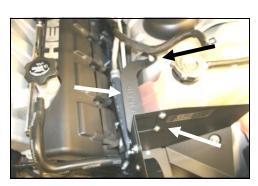
12. Install the rear support bracket (#6) from the **CAD** to the inner fender using three  $\frac{1}{4}$  - 20 x 1/2" button head bolts (#13),  $\frac{1}{4}$ " flat washers (#14), 1/4" serrated nuts (#15), and the 10mm factory nut removed in step #11.
