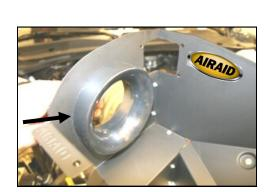
**8.** Next, install the filter adapter (#5) using three  $\frac{1}{4}$  - 20 x 1/2" button head bolts (#13), and  $\frac{1}{4}$  flat washers (#14).
