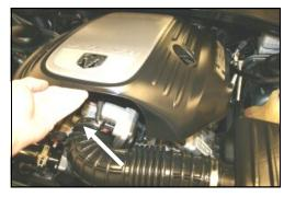
**1. Disconnect the negative battery cable.** *If you are working on a 5.7L, first remove the engine beauty cover by lifting it up off of the grommets.* Next, loosen the hose clamp that holds the factory intake tube to the throttle body.
