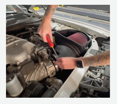
Reinstall the stock screw at the front of the vehicle.
