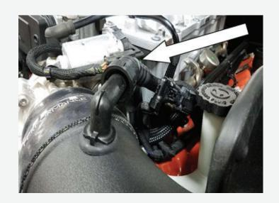
Unfasten the two screws holding the coolant tank to allow for more room when removing the stock intake and installing the JLT intake.
