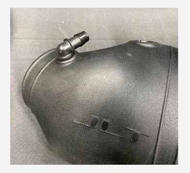
Care fully remove the IAT sensor from the stock tube. Then, install the supplied IAT grommet and the previously removed IAT sensor into the JLT tube by twisting it so the tab is as shown.
