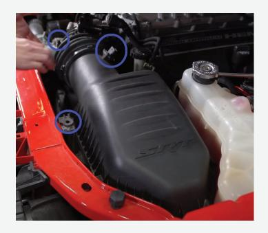
If you have a vehicle like the image to the right, cut the corrugated hose coming from the stock intake at the end connected to the vehicle, being careful to not damage the barbs on the fitting. Alternatively, you can also heat it up using a heat gun so it remains intact instead, being cautious to not heat up other components in the same area.
