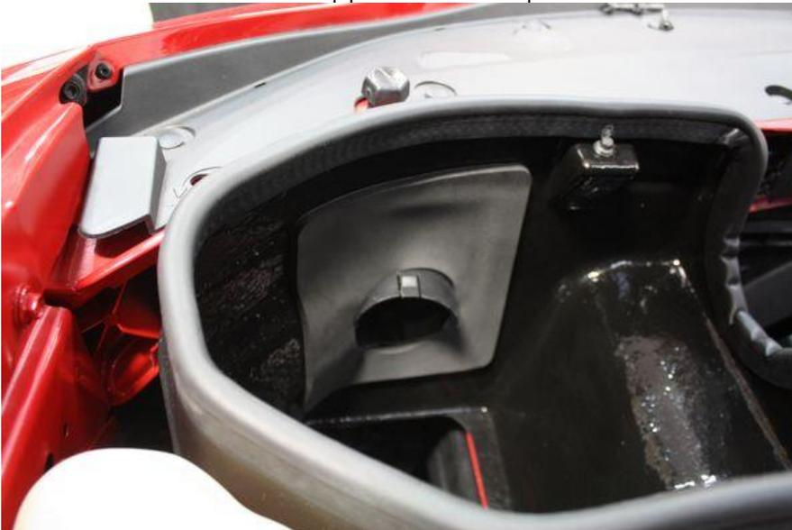
8 Remove from factory intake: MAF or IAT sensor(Twist to unlock), PCV connection
